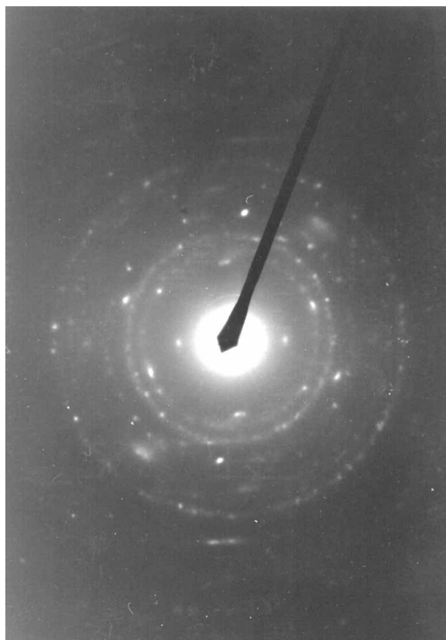
Figure 3(b). Shows a SAD pattern, approximately 0.1 mm in diameter taken from a region in Fig. 1, containing a variety of crystals including one large lath-shaped crystal. Superimposed on the spotty ring-type pattern that is similar to that in Figure 2(a) is a partial single-crystal pattern. The prominent row of spots for this pattern has a spacing corresponding to 10.7 Å which is consistent with tochilinite.
