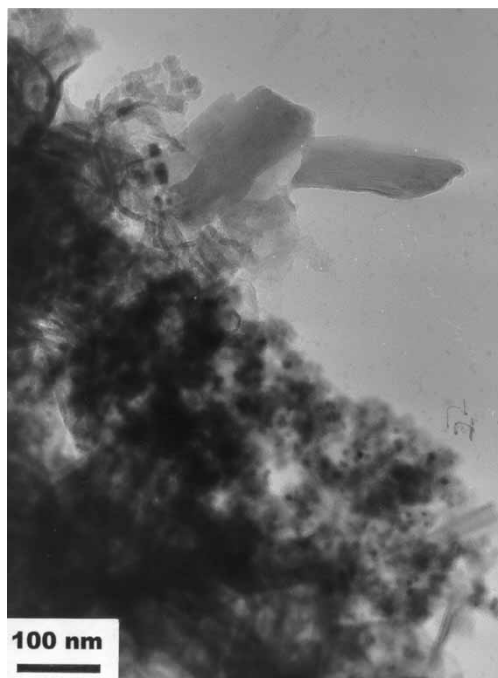
Figure 1. Shows that the adsorbent contains two distinct crystal morphologies. Small rhombs, as shown at higher magnification in Fig. 2(a), mostly between about 10 nm to approximately 30 nm across wide and curling lath-like particles up to about 5–10 nm wide and 50–100 nm long, but occasionally larger, irregular-shaped crystals occur up to about 100 nm wide and 200 nm long.
